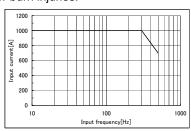
Figure 1. Permissible current to frequency
